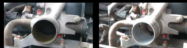
BEFORE (Throttle body condition after 60,000 km)
